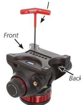
**6.** Take the replacement bridge and re-install the 4 hex screws that were removed in Step 2 with the 4MM hex wrench. **Please note: Still keep the Manfrotto Fluid head lock knob and drag knob in the locked position. Make sure that the replacement bridge has the front to the front and the back to the back.**
