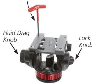
**2.** Start by fully locking the fluid head lock knob and fluid drag knob. Now take enclosed 4MM hex wrench (B) and remove the 4 hex screws holding the original Manfrotto bridge.
